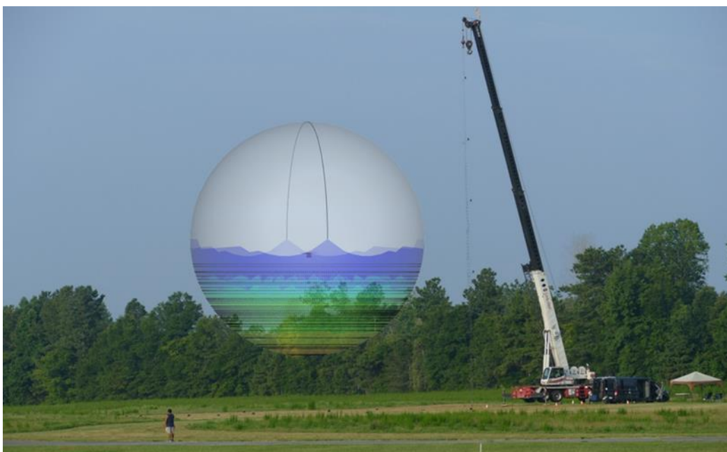
Figure 2 – Measurement of hexacopter drone by microphones suspended from a crane and along the ground with the noise directivity pattern superimposed on drone location shown by the colour contours on the transparent sphere.
